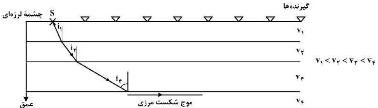
$$\sin i_1 = \frac{v_1}{v_4}, \sin i_2 = \frac{v_2}{v_4}, \sin i_3 = \frac{v_3}{v_4} \quad (۲) \qquad \sin i_1 = \frac{v_1}{v_2}, \sin i_2 = \frac{v_2}{v_3}, \sin i_3 = \frac{v_3}{v_4} \quad (۱)$$
